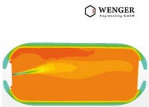
The aim of the project was to better understand and optimize a 700-bar hydrogen tank using CFD simulation. The main focus was on local temperatures during refuelling and cooling during fast de-fueling.
